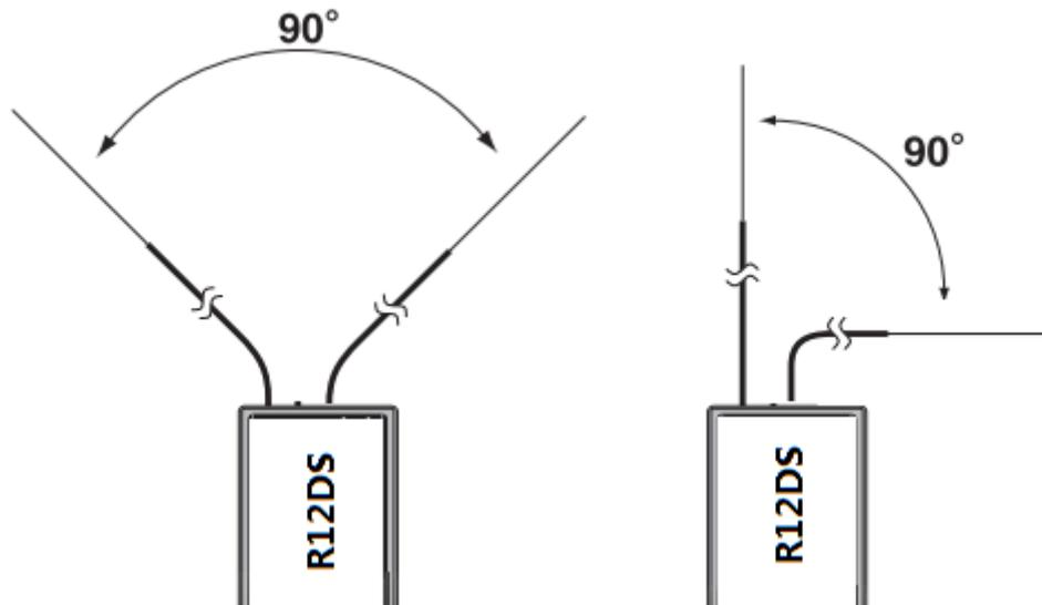
3. Large model aircraft may have some metal part interfering signal; in this case the antennas should be placed at both sides of the model. Then the best RF signal condition is obtained at any flying attitude.
