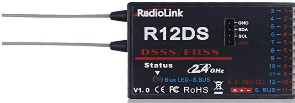
Radiolink R12DS, 2.4G 12 channels receiver, DSSS and FHSS spread spectrum working synchronously, compatible with Radiolink transmitters AT9, AT9S, AT9S Pro, AT10 and AT10II(AT9, AT9S, AT10 can upgrade to 12 channels just upgrade by firmware, you can download the firmware from our website: [www.radiolink.com](http://www.radiolink.com) AT10II is default 12 channels).
